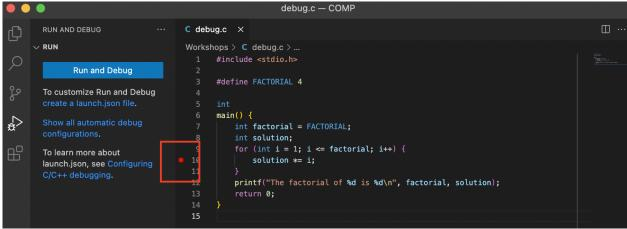
7. When you "Run and Debug" the program stops at the breakpoint. Note the Variables presented in the top left and their live values. We may already notice an issue, before line 10 is run (the current line is highlighted in yellow), the value for the solution is 3.
